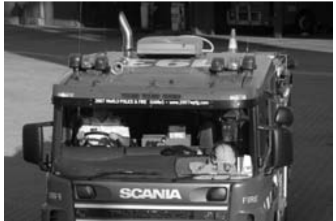
Pumping Appliance with the Air Conditioning Unit on the roof
